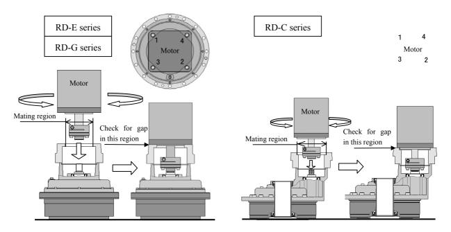
$<sup>\</sup>Rightarrow$ Secure the servo motor to the gear head using the Allen bolts. Tighten the opposing side bolts evenly to the tightening torque designated by the servo motor manufacturer.
